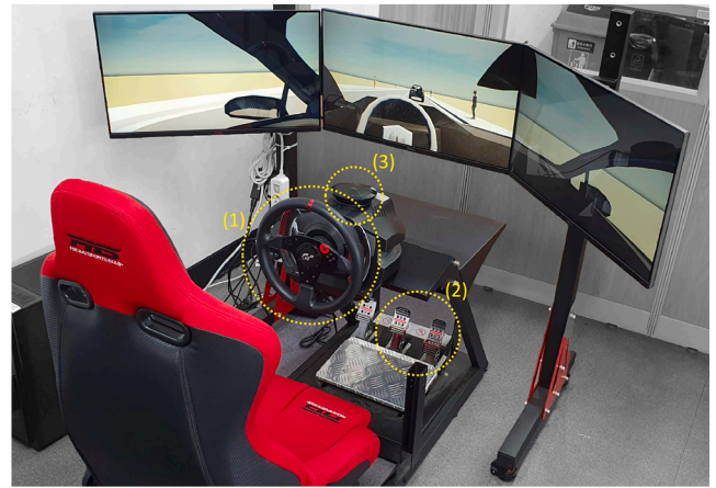
Fig. 1. L2 automated vehicle simulator with a cockpit module: (1) a steering wheel; (2) a brake pedal; (3) a speakerphone.
